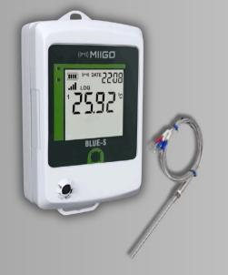
MIIGO BLUE-S-B-RTDX + MI-RTDX SENSOR Ultra high-accurate RTD datalogger with (PT100, PT1000, DIN 1/10, 1/5, 1/3) sensor with 40K memory, High-speed logging (1sec to 24 hrs), Audible + Visual Alarms, 10-point drift-adjustment / calibration feature [Real-time monitoring over Mobile/PC Application]
