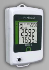
MIIGO BLUE-S-B-THI: Humidity Temperature Datalogger with Ulta High Accuracy of ± 1% RH, ± 0.2 °C, Resolution - 0.01 %RH / 0.01 °C. Ideal for Thermal Mapping /validation. with 60K memory, High-speed logging (1 sec to 24 hrs), Audible + Visual Alarms, 10-point drift-adjustment / calibration feature [Real-time monitoring over Mobile/PC Application]
