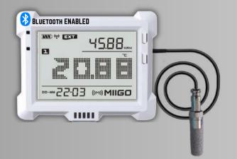
MIIGO BLUE-H-A-THE + MO-RHX Sensor (MAX 3 METER CABLE): %RH-Temp Data Logger (EXTERNAL SENSOR) with Ulta High Acc. of ± 1% RH, ± 0.2 °C, Res. - 0.01 %RH / 0.01 °C, 60k memory, 1 sec to 24hrs high-speed login, Audible + Visual Alarms, 10-point drift adjustment & calibration feature [Real-time monitoring over Mobile/PC Application]
