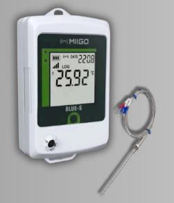
MIIGO BLUE-S-B-RTDX + MI-RTDX SENSOR Ultra high-accurate RTD datalogger with (PT100, PT1000, DIN 1/10, 1/5, 1/3) sensor with 40K memory, High-speed logging (Isec to 24 hrs), Audible + Visual Alarms, 10-point drift-adjustment / calibration feature [Real-time monitoring over Mobile/PC Application]
