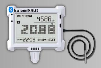
**MIIGO BLUE-H-B-THIT1 + MI-DTC Sensor:** Digital Thermo Hygrometer with Ulta High Accuracy of  $\pm 1\%$  RH,  $\pm 0.2$  °C, &  $\pm 0.3$  °C (Ext Temp Sensor). Resolution – 0.01 %RH / 0.01 °C / (0.1/0.01), 60 days stat memory, 15 alarms on display (FIFO), Audible + Visual Alarms, 10point drift-adjustment & calibration feature [Real-time monitoring over Mobile/PC Application]
